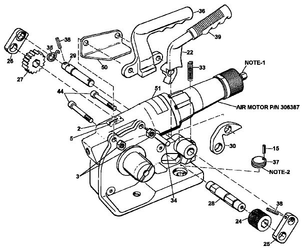
NOTE 1. Use large quick disconnect fittings: Socket P/N 0200706, Plug P/N 020704 NOTE 2. Assemble wear pad with "B" side down.
