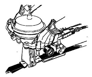
If for some reason the gripper will not energize, do not try to energize using the pawl handle, as this will result in disengagement of the ratchet wheel. Apply light machine oil to the pivot pin (5), until the lever moves freely.
