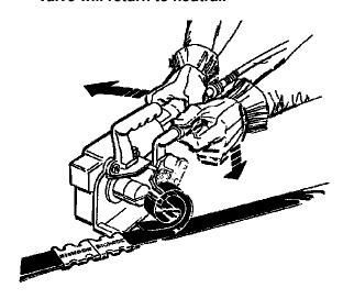
Lift the pawl handle thereby disengaging the ratchet wheel. Then press down on the pawl handle and rotate the tool off the strap in a counterclockwise direction.
