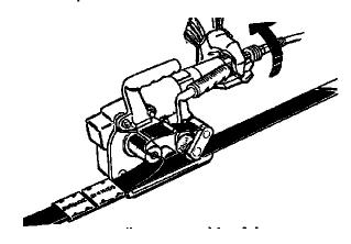
While standing to one side of the strap line, rotate the valve collar clockwise to tension strap allowing motor to stall out at desired tension.
