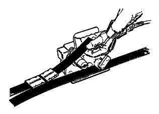
Thread strap in to the windlass and under the strap pin. Strap should extend 4" - 8" beyond the windlass.
