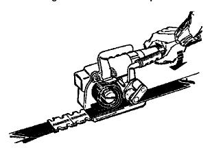
8. After sealing the strap, rotate the valve collar counterclockwise to unwind the windlass. Note tab end of strap in windlass. When this becomes loose, the tool will be easily removed. The valve collar is spring loaded to the reverse direction so that when released, the valve will return to neutral.
