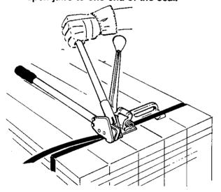
2. Bring the sealer handles completely together to assure a proper notch.
