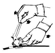
Hold sealing tool at right angles to strap, resting it squarely over seal. Seal the tensioned strap by bringing sealer handles together as far as they will go.
