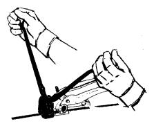
Return tensioning handle to rest on the tool by pressing the handle pawl with thumb. Squeeze handle to base and remove tool from strap by swinging rear foot out, as illustrated.
