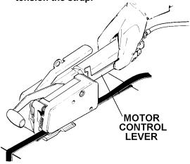
3. When the motor stalls, indicating completion of tension, <u>continue to hold</u> <u>the motor lever fully closed</u> against the motor housing and pull back the weld handle with your left hand. The handle should be pulled <u>quickly</u> all the way back without hesitation. When the weld lever is pulled back it traps the motor lever in the <u>ON</u> position.
