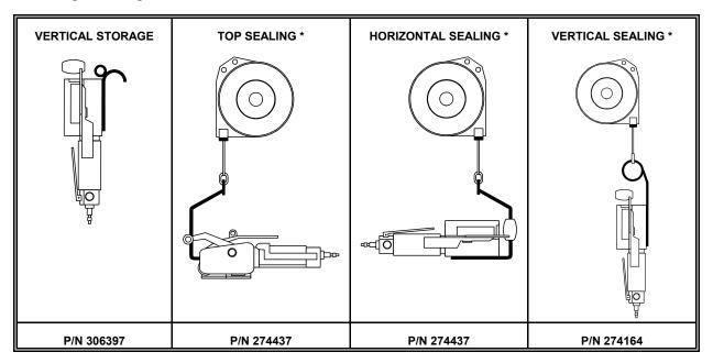
\* Shown with the recommended Overhead Tool Balancer, Signode Model Number P-5602.
