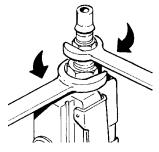
AIR MOTOR VALVE Remove the air valve as follows:
