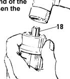
11. Disassemble the rotor by sliding off the front end plate (20), and any ball bearing(s) and spacers. Then slide the back end plate (14) and the rotor assembly (18), with the vanes (17), out of the cylinder.
