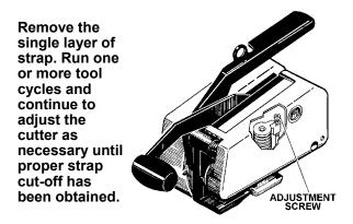
NOTE: Do not over tighten cutter mechanism as lower strap damage or poor strap cut-off will occur.
