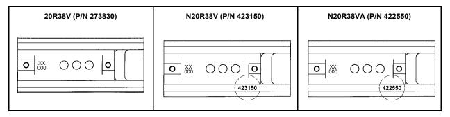
NOTE: Air motor 20R38V is an older style air motor used on VXL/VXM tools. Air motor 20R38V can be identified by the absence of a part number engraved or stamped on the underside of the motor housing.
