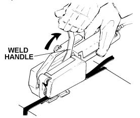
4. The internal weld timer is energized. The strap is welded and the supply end of the strap is cut-off. Pull the cut strap away during welding. The tool will continue through the weld cycle and stop with the motor lever being held in place. When the timer times out, the weld action stops. Allow the tool to remain stationary for at least 3 seconds to ensure that the weld is fully cooled.
