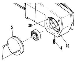
INSERT 2 #10-24 SCREWS, (NOT PROVIDED), INTO END CAP TO ASSIST IN REMOVAL FROM HOUSING.
