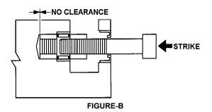
With the gear housing firmly braced, strike the end of the screw firmly with a hammer to drive the bearing into the spacer. This action will prevent the spacer from rotating while screw is threaded in.
