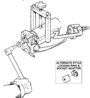
NOTE: If disassembling a tool with the alternate style locking ring, use socket adapter Part No. 422341.
