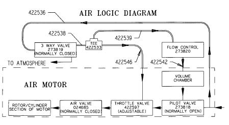
motor starts running again. Air flows through the 3-way valve, the flow control and enters the volume chamber. When sufficient pressure has built up in the volume chamber the pilot valve will actuate and shut off the air flow to the air valve and the rotor/cylinder. The air motor then stops.
