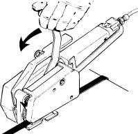
6. Press the operating lever and swing the tool off the strap, rear of tool first. Inspect the joint to make sure the straps have been properly welded.
