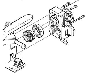
5. Remove the locking ring from the motor mount. NOTE: The locking ring has left-hand threads.
