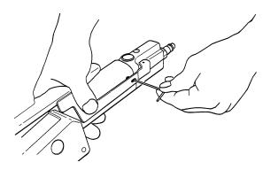
NOTE: Operating air pressure must be set between 85 and 90 psi (5.7-6.2 Bar). With accurately controlled air pressure the tension will be uniform on all straps, provided the operator allows the air motor to stall. This kit contains the following items:
