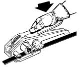
3. Fully insert the upper strap into the slot of the cutter mechanism and the windlass.
