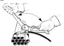
4. When desired tension is reached, push the drive pawl forward and rotate the tension handle back to contact the lift arm.
