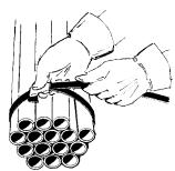
Squeeze the handles together to lift the feedwheel. Insert the strap into the slot of the breaker nose and push the tool up against the seal.
