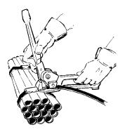
Notch the seal with a Delta sealer to complete the joint.
