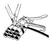
Break off the strap at the seal by raising the tool perpendicular to the seal, then lowering it.
